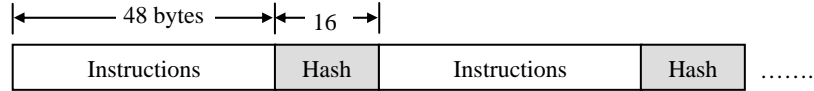
Figure 4: Instruction stream of the trusted module with integrity hashes inserted at the cache line boundary, assuming 64-byte cache line.
