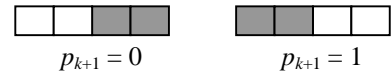
Figure 5. Bits selected from the i th 4-bit subword of rs by sieve in 2-bit mode
