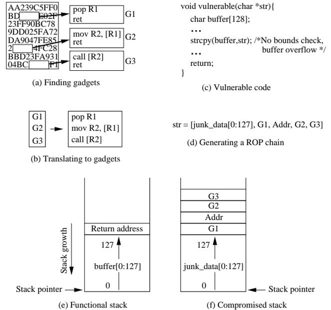
Figure 10: Example of Return Oriented Programming attack.
