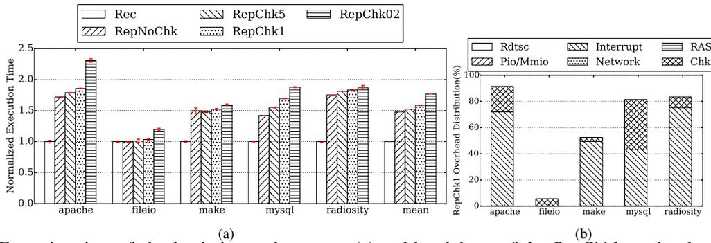
Figure 8: Execution time of checkpointing replay setups (a) and breakdown of the *RepChk1* overhead over *Rec* (b).
