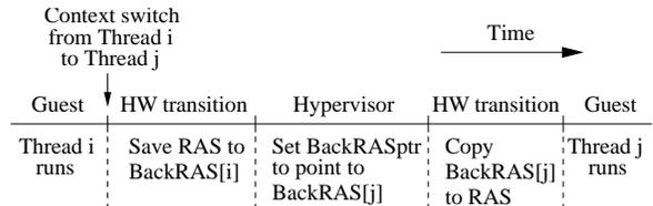
Figure 3: Algorithm and timeline to handle multiple threads.
