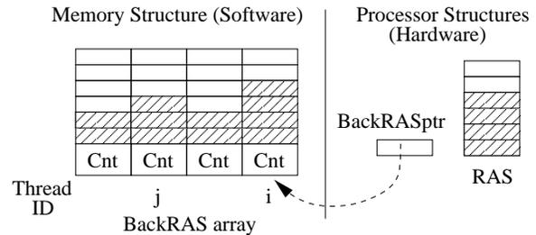
Figure 2: Structures used to support multiple threads.
