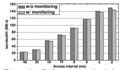
Figure 15: Performance overhead for monitoring disk attacks
