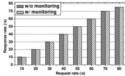
Figure 14: Performance overhead for monitoring network attacks
