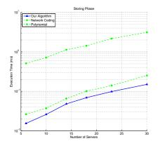
Figure 6: Compare the total execution time for storing phase. Our algorithm exhibits minimum execution time of 0.1ms for n = 20servers, since it only needs bitwise XOR operation and pseudorandom vector generation. Algorithm 1 for storing phase is very efficient.
