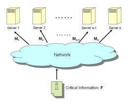
Figure 1: This figure shows the storage of a piece of critical information, denoted by  $\mathbb{F}$ , on *n* distributed servers over a network.
